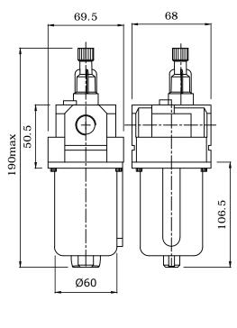
Supply pressure 6 bar , pressure drop p= 0.5 bar (for standard models)
